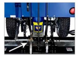
Advanced Water System — AWS<sup>™</sup> Regulates the amount of water dispensed onto the ice relative to the machine speed for an efficient and even application.
